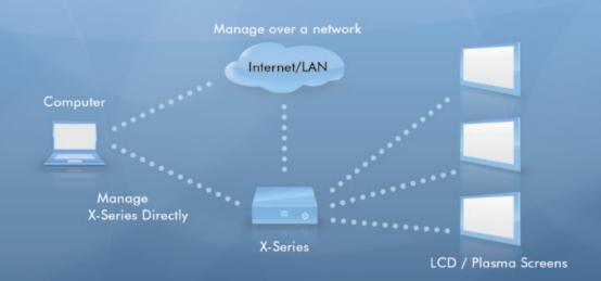
Connect the X-Series Digital Signage Engine to a local network or the Internet and directly to a display. Networked systems allow users to reach the X-Series' content management system via a web browser. The device includes tools for easy system administration.
